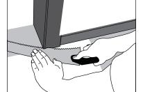
(2) Door molding and skirting: lay a board (with the decorative side down) next to the door molding and cut as shown in the figure. Then slide the floorboard under molding.
