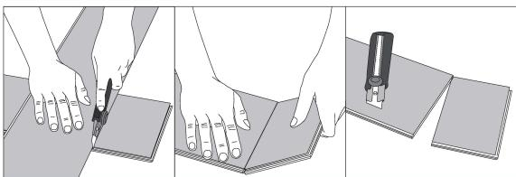
(5) To cut the plank, use a simple utility knife and ruler, and with the top side facing up, cut heavily and several times on the same axis. The knife will not go through the surface but make a deep cut. You can then lift one half of the plank using your other hand to hold
