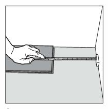
4 At the end of the first row, leave an expansion gap of 1/4" to the wall and measure
