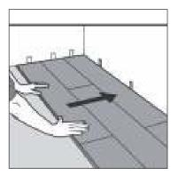
(9) After 2-3 rows. Adjust the distance to the front wall by leaving an expansion gap of 1/4". Always ensure that the end joints are staggered at least 8", both when in the same row as when from one row to the next one.
