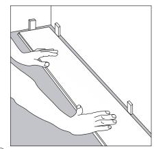
(1) After thoroughly cleaning the subfloor, you should begin laying in the left-hand corner. Place the floorboard 1/4" from the left wall. Use spacers between the wall and the floorboard.
