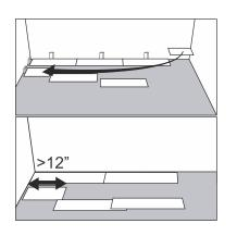
(6) Start the second row with the leftover cut part of the last plank of the previous row. This small plank should measure at least 12". Otherwise, use another plank that should be cut in two. The end joints of each adjoining row should not be closer than 8" to each other.
