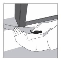
(12) Door molding and skirting: lay a board (with the decorative side down) next to the door molding and cut as shown in the figure. Then slide the floorboard under the molding.
