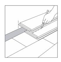
(10) To lay the last row: position a loose board exactly on top of the last row laid. Place another board on top, with the tongue side touching the wall. Draw a line along the edge of this boards, to mark the first board. Cut along this line to obtain of the required width. Insert this cut board against the wall. The last row should be at least 2" wide. The spacers can then be removed.
