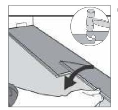
(2) Second Plank, first row. Drop the plank and gently press down the end with a rubber mallet so it firmly locks into the previous plank until both are at the same height. Make sure both planks are perfectly aligned. NOTE: If you notice both planks aren't at the same height or are not well locked together, please follow the disassembling instructions at the bottom of the page, disassemble and check if any debris stuck inside the lock is obstructing.
