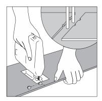
(1) Holes for pipes: measure the diameter of the pipe and drill a hole that is 7/8" larger. Saw off a piece as shown in the figure and lay the board in place on the floor. Then lay the sawed-off piece in place.
